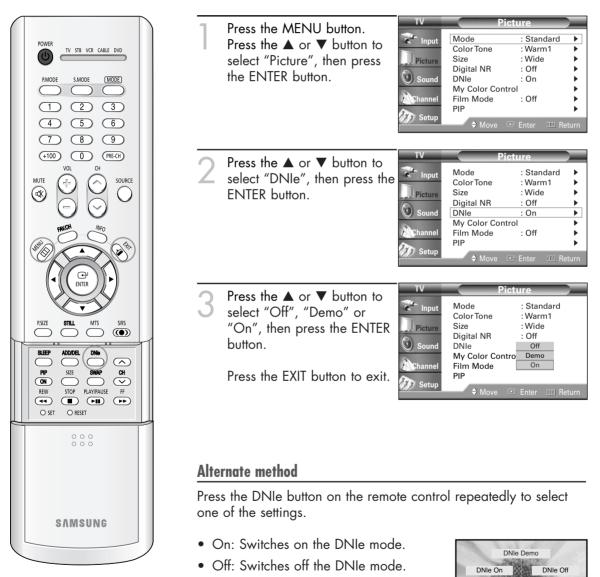
• Demo: The screen before applying DNIe appears on the right and the screen after applying DNIe appears on the left.
